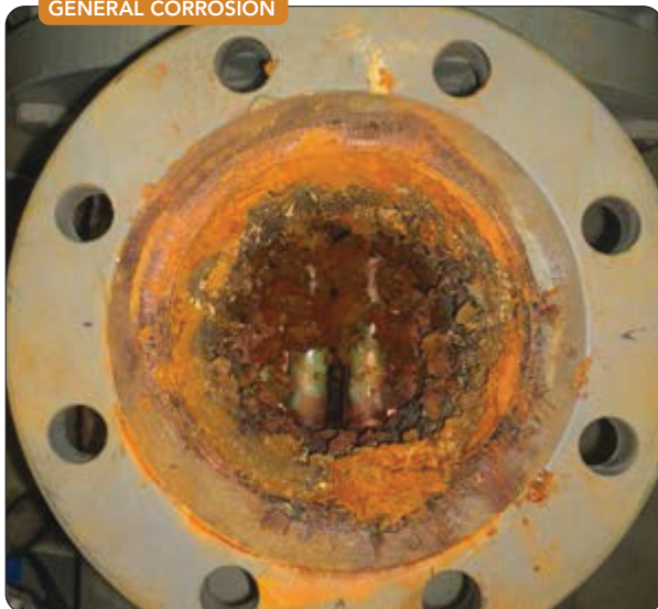
Figure 1. This usually involves a relatively uniform attack over a surface, often without evidence of its occurrence.
