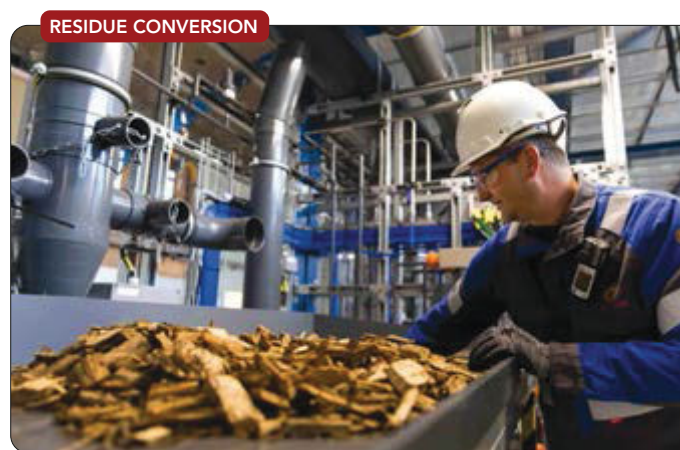
Figure 2. Proprietary technology produces industrial sugars and lignin from forestry and agricultural residues at pilot biorefinery. Source: Avantium.
