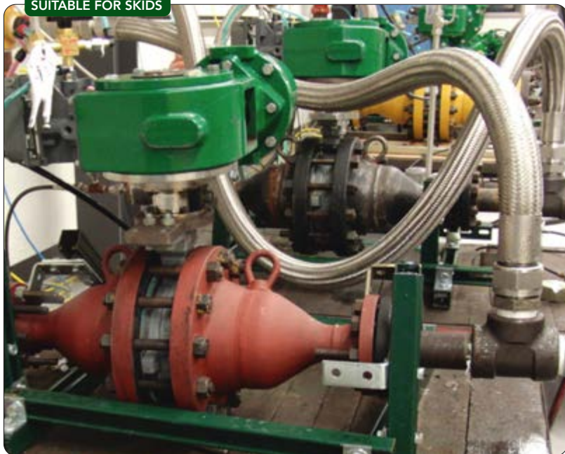
Figure 2. Valves must be compact to fit on the skid of a PSA unit.
