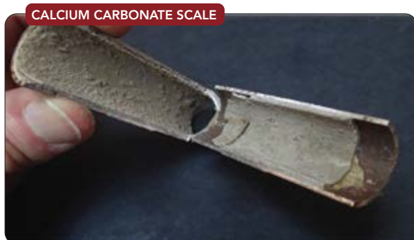
Figure 1. Precipitation from water can cause buildup on internal surface of heat exchanger tube.
