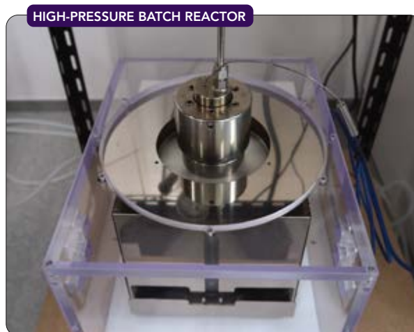
Figure 2. Reaction takes place at a lower temperature than needed by other plastics conversion processes. Source: Osaka City University.
