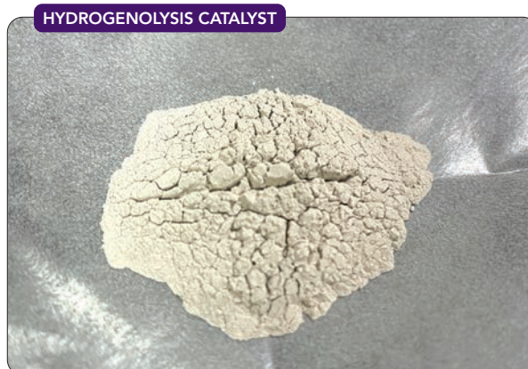
Figure 1. Platinum/metaphosphate catalyst spurs production of arenes from phenols at mild conditions. Source: Xiongjie Jin/University of Tokyo.
