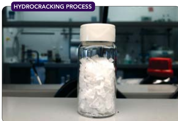
Figure 1. Low-temperature treatment breaks down shredded plastic into smaller carbon molecules used to create jet fuels, diesel and lubricants. Source: University of Delaware.
