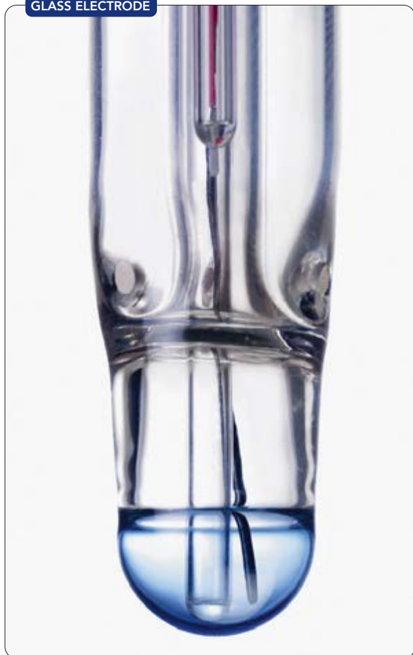
Figure 2. The pH sensor contains an aqueous internal filling solution of a known pH along with a coated silver wire called an internal element.
