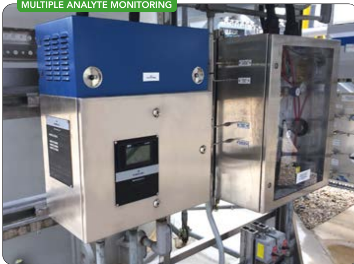
Figure 3. A hybrid QCL/TDL analyzer, such as Emerson's Rosemount CT5100 Continuous Gas Analyzer, can contain up to six laser modules, some of which can measure two analytes.
