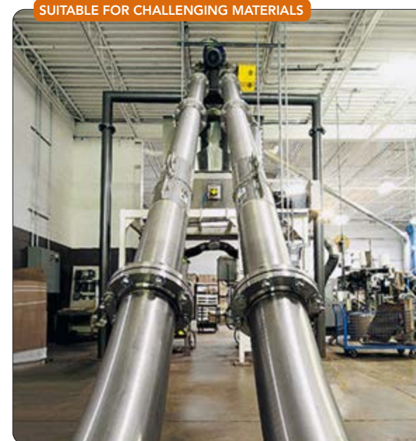
Figure 1. This 8-inch tubular drag conveyor elevates product into hopper for packaging.
