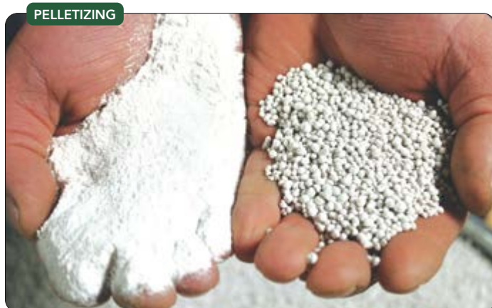
Figure 3. Fine material (left) is turned into larger, refined pellets (right) by this technique.
