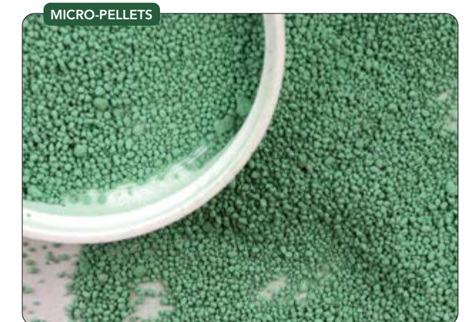
Figure 2. A pin mixer, because of its intense spinning action, yields small, dense pellets.
