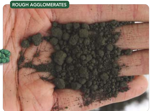
Figure 1. Conditioning, which can produce such agglomerates, often provides a quick and straightforward option for de-dusting.
