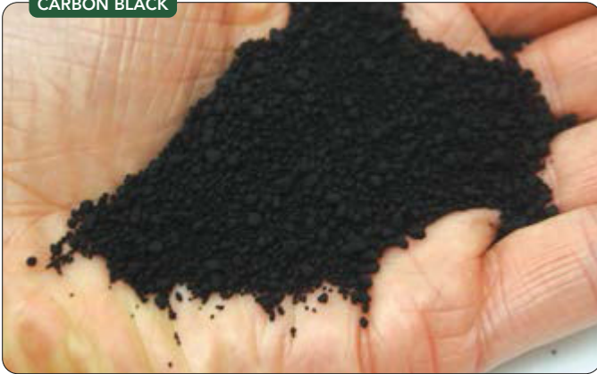
Figure 4. Manufacturers of the material long have relied on agitation agglomeration to increase particle size and improve handling and safety.
