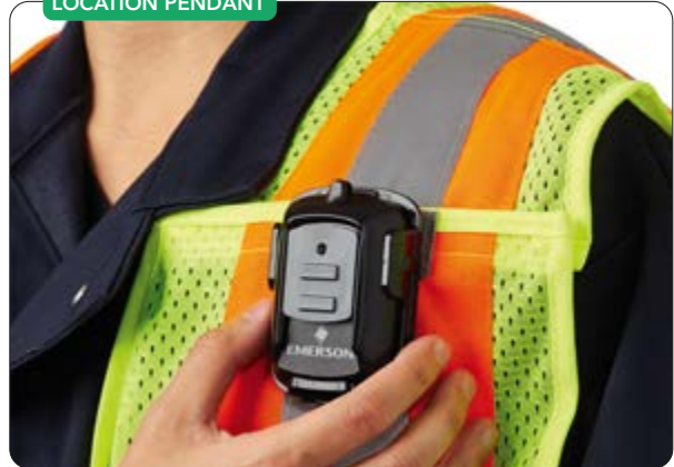
Figure 3. Pushing a button enables a worker to signal an injury or emergency as well as the person's location.
