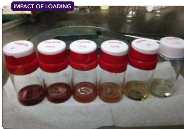
Figure 2. The amount of the white solid polynorbornene produced varied with catalyst loading. Source: OIST.
