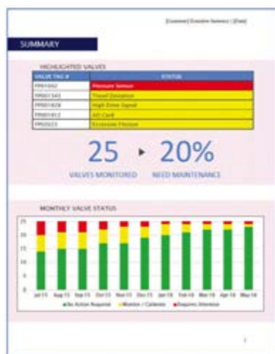
Figure 4. Outside experts can monitor valve diagnostic data and highlight developing problems as well as serious issues demanding immediate attention.
