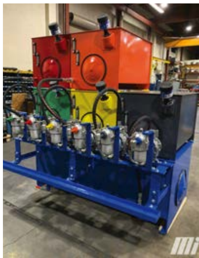
Figure 1. Built by one of Motion’s Service Centers, this oil storage system was designed for plant maintenance, featuring highly organized placement and color-coding. The unit type shown is universal and applicable in all kinds of industries, including chemical processing—and can be customized to handle the proper fluid types for the application.
