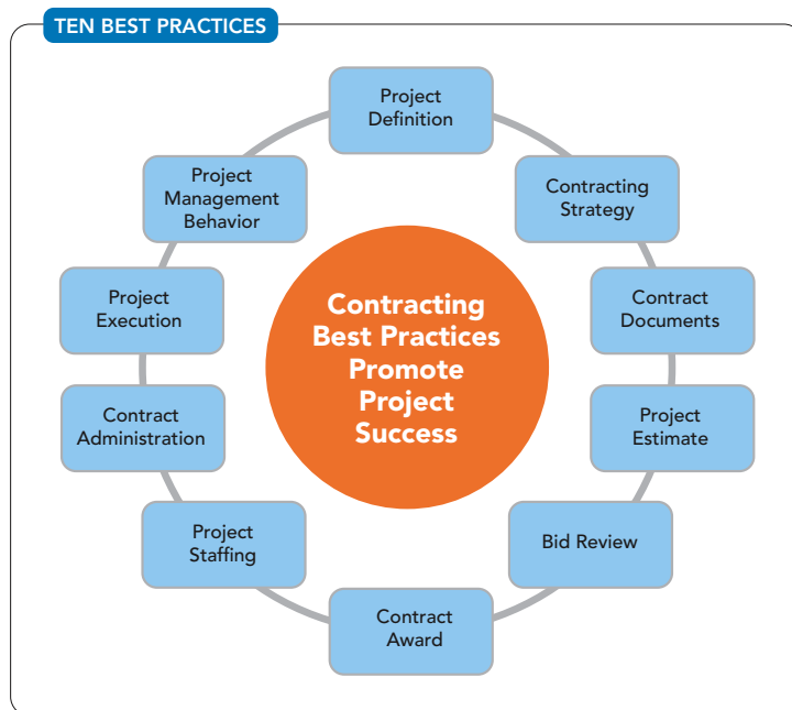
Figure 2. These can head off common contracting errors.
